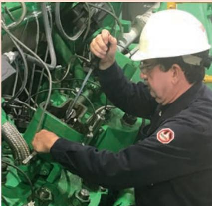
**An employee performs maintenance work on a 12Q145-H Cooper-Bessemer integral engine-compressor. With the Arcline purchase of BHGE's reciprocating compression division, the new standalone company has chosen to operate as Cooper Machinery Services.**
